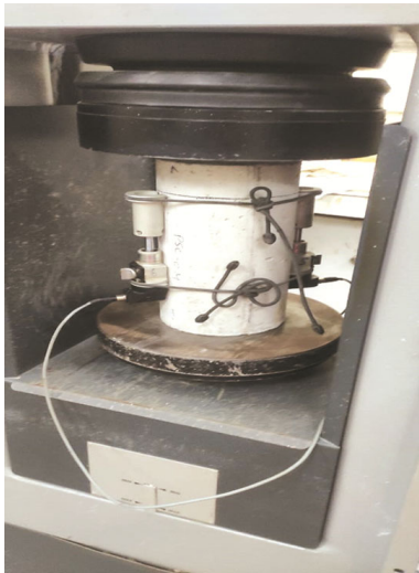
Fig. 2 — Test setup for Modulus of Elasticity of SCC mixture.
