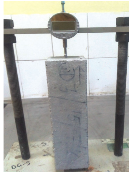
Fig. 3 — Test setup for drying shrinkage of SCC mixture.
