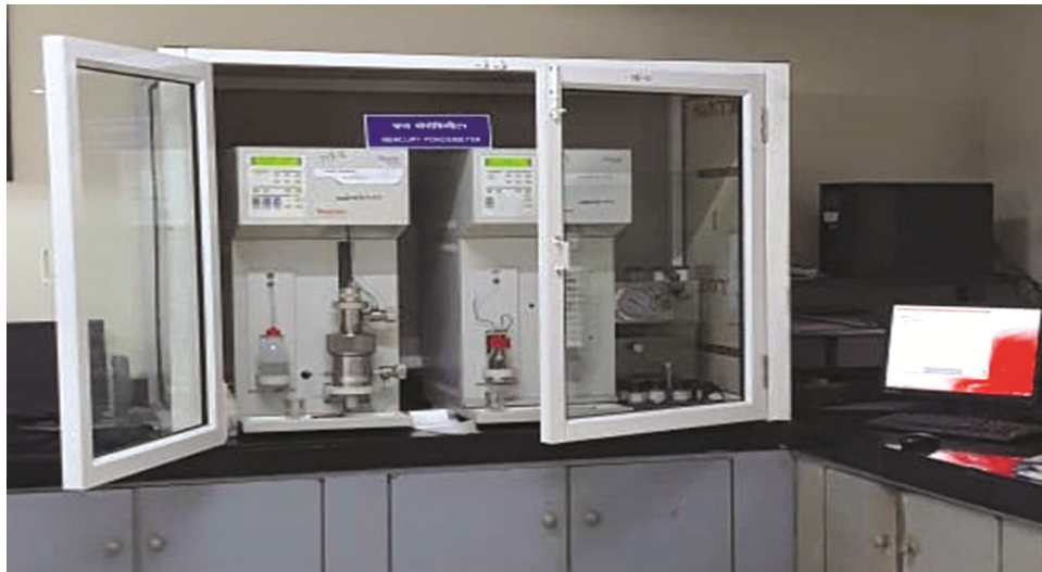
Fig. 10 — Test setup for Mercury intrusion porosimetry of SCC mixture.
