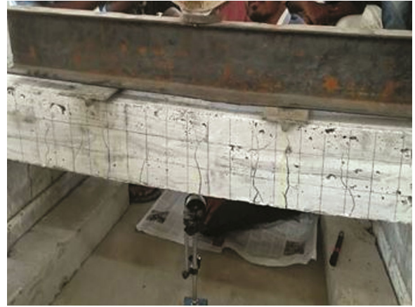
Fig. 2 — Flexural cracks formation and propagation during the experiment.
