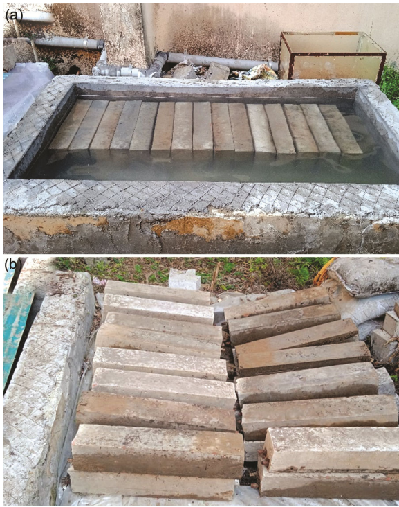
Fig. 5 — (a) beam samples in 5% NaCl solution, and (b) drying phase. (wetting cycle). Figure 5b shows the beam samples in the drying phase.
