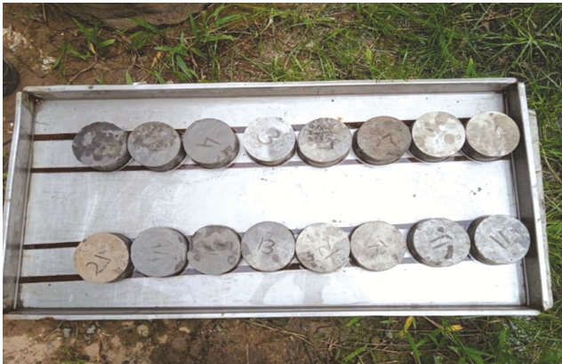
Fig. 2 — Sorptivity test setup.
