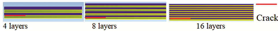
Fig. 8 — Position of the crack at bottom layer of the laminate at the left end (Position C).
