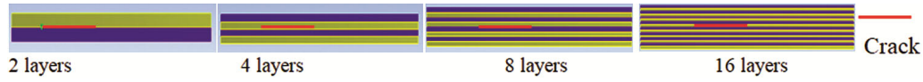
Fig. 7 — Position of the crack at 15mm away from left end of center layer of the laminate (Position B).
