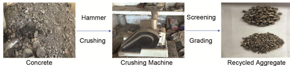
Fig. 2 — Manufacturing process of recycled concrete aggregate.
