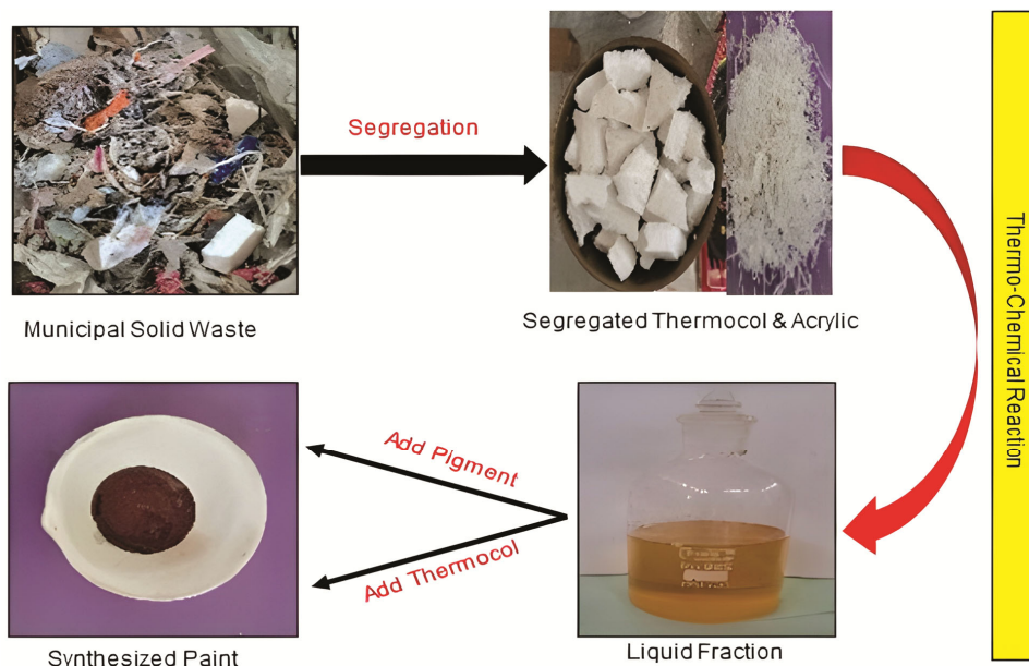
Fig. 5 — Paint Preparation Procedure.
