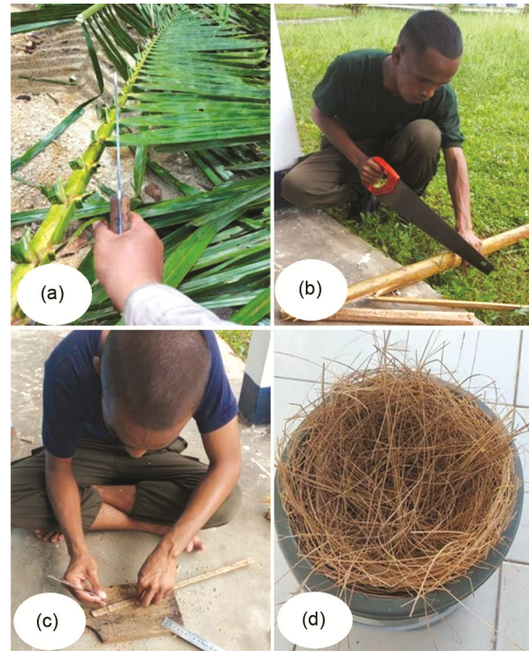
Fig. 4 — The process of obtaining sago midrib fiber material; a) Separation of the leaf from the midrib; b) Cutting the sago midrib; c) Separation of pith with fiber; and d) sago midrib fiber
