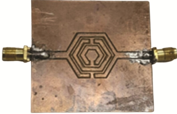
Fig. 2 — Fabricated two-port H-SRR sensor with SMA connectors.
