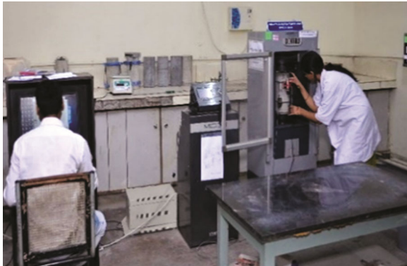
Fig. 1 — Test set-up for compressive strength.
