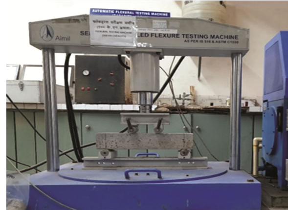
Fig. 2 — Test set-up for flexural strength.
