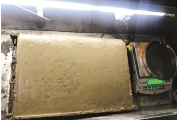
Fig. 10 — Plastic shrinkage test on AAC mix.
