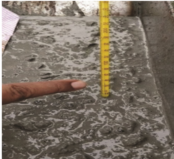
Fig. 12 — Temperature measurement of AAC mix.
