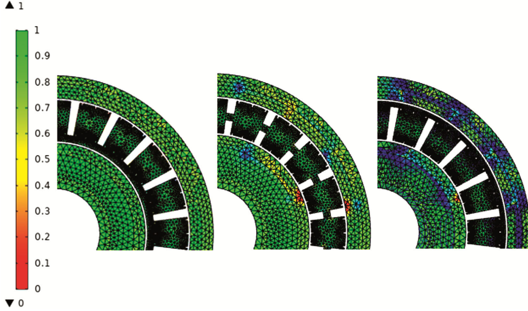
Fig. 11 — Mesh quality by using skewness for the above three modulator bridge configurations.
