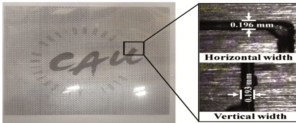
Fig. 6 — Optically transparent absorber fabricated on a PET sheet using inkjet printing 46 .
