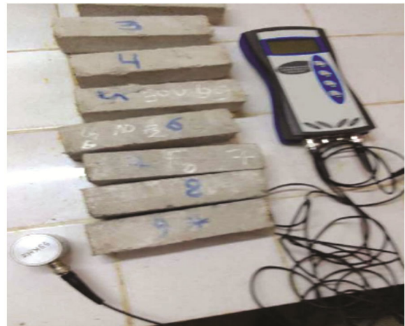
Fig. 3 — PUNDIT apparatus, in accordance with the NF EN 12504-4 standard.
