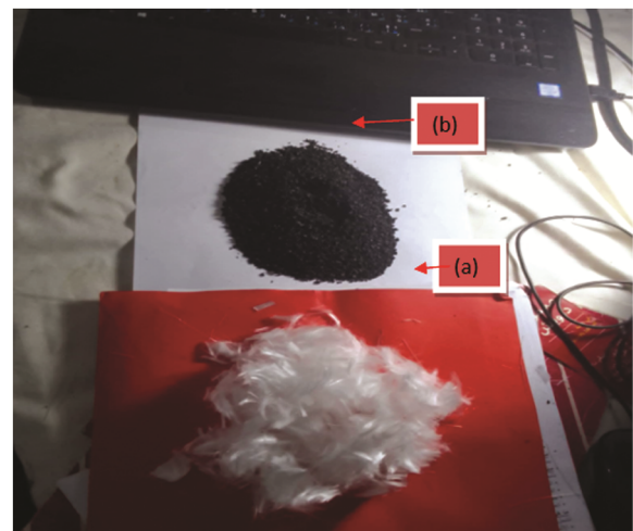
Fig. 1 — Photographic view of the materials used (a) polypropylene fibers, and (b) recycled rubber aggregates.
