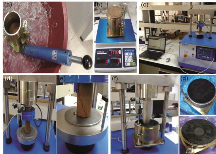
Fig. 6 — (a) and (b) Applications of the experimental tests, (c) and (d) Standard proctor test, (e) Unconfined compression test, (f) and (g) CBR test.
