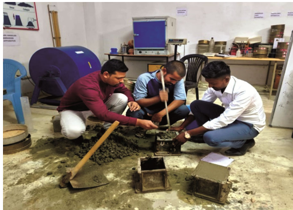
Fig. 1 — Preparation of mix design sample in concrete laboratory.
