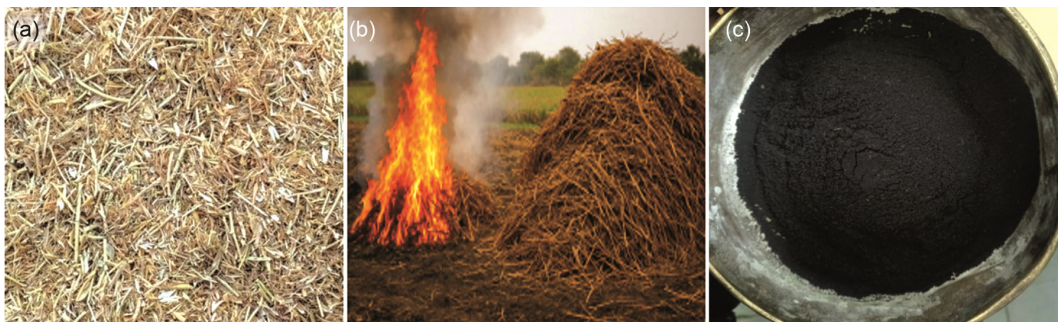
Fig. 1 — (a) Wheat husk pile, (b) Ash generation by burning (c) Wheat husk ash.
