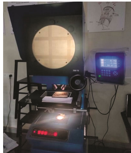
Fig. 2 — Optical profile projector showing the workpiece mounted on bed with magnified kerf.
