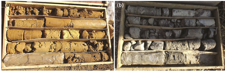
Fig. 8 — Display of boxes from core surveys SC02(a)The coring campaign at a depth between 0.00m and 5.00m, and (b)The coring campaign at a depth between 5.00m and 20.00m.
