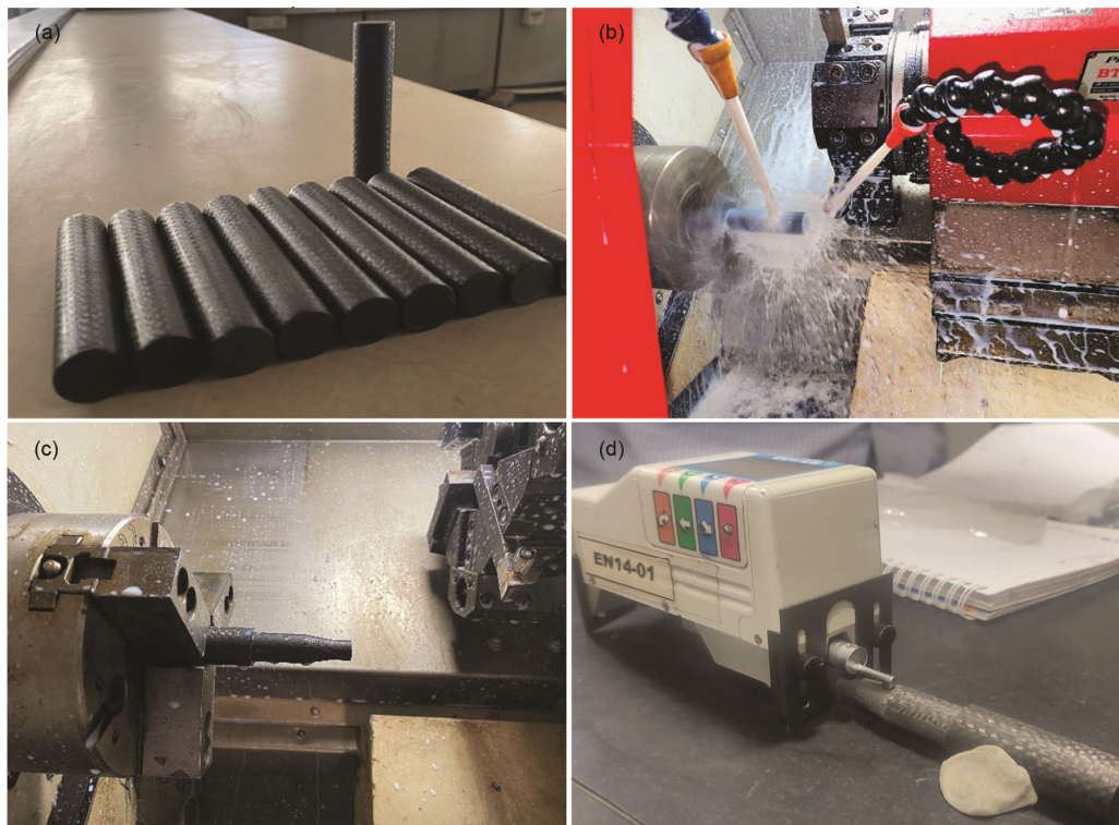
Fig. 2 — (a) 3K CFRP material (HSN CODE-68151200), (b) Turning of CFRP under 3 bar coolant pressure, (c) Finished Component and (d) Measuring the surface texture (Ra).
