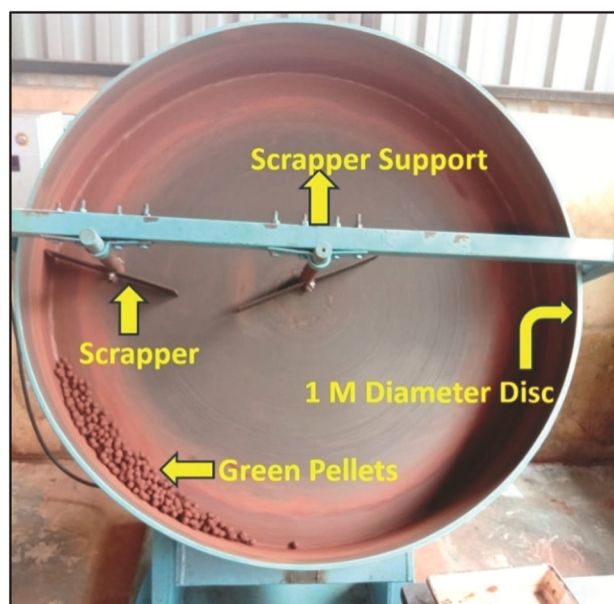
Fig. 2 — Picture of laboratory scale disc pelletizer used in the study [Disc Diameter- 1m; Disc Inclination- 47°; Disc Rotation- 20 RPM].
