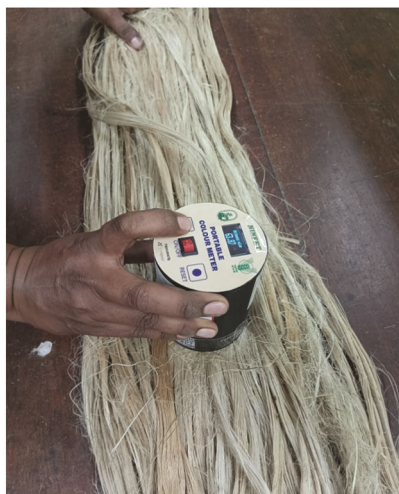
Fig. 4 — Testing of colour meter.
