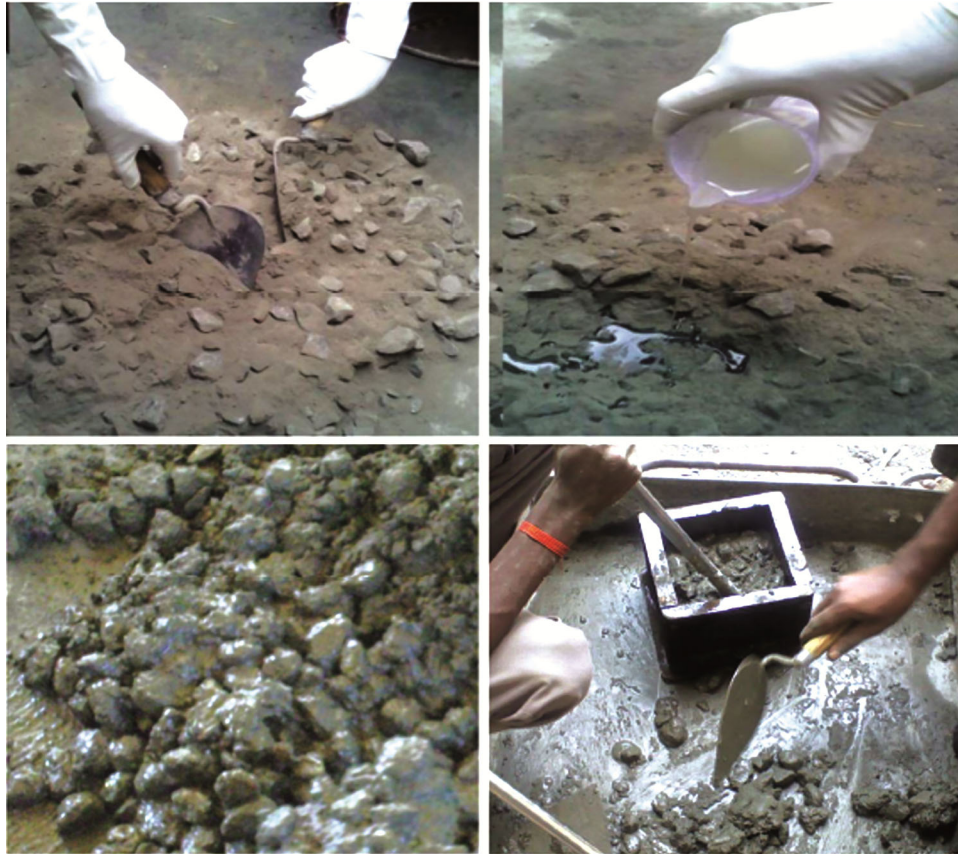
Fig. 5 — Casting and mixing of GPC samples.
