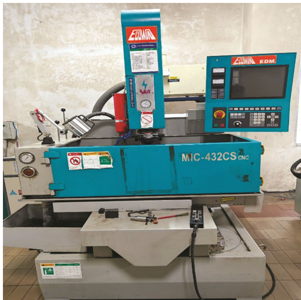
Fig. 1 — CNC-EDM Machine (Model: MIC 432CS, ECOWIN, Taiwan).
