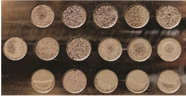
Fig. 2 — Machined workpiece EN-40 alloy steel.
