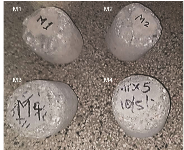
Fig. 6 — Abraded surface of different concrete mixes after Cantabro abrasion test.
