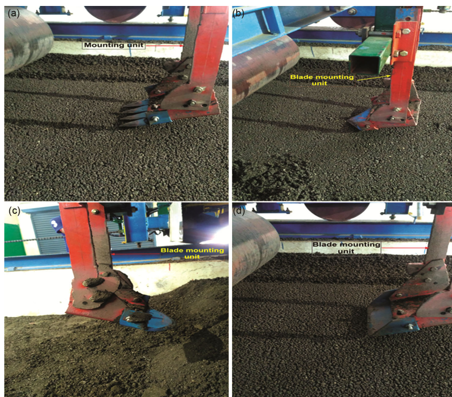
Fig. 2 — Different shape of blade attached with the mounting unit in soil bin (a) V shape, (b) triangular fork, (c) convex and (d) rectangular.
