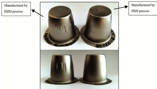
Fig. 15 — The sample conical industrial parts that were formed with both hydromechanical deep drawing (on the left) and DSH process.
