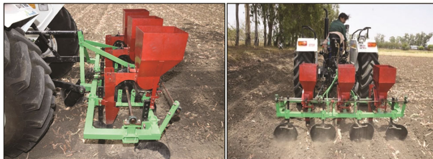
Fig. 16 — Developed ginger planter in field operation.
