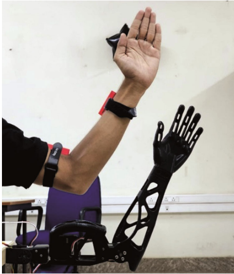
Fig. 2 — Designed human collaborative humanoid robotic hand controlled using sensors.
