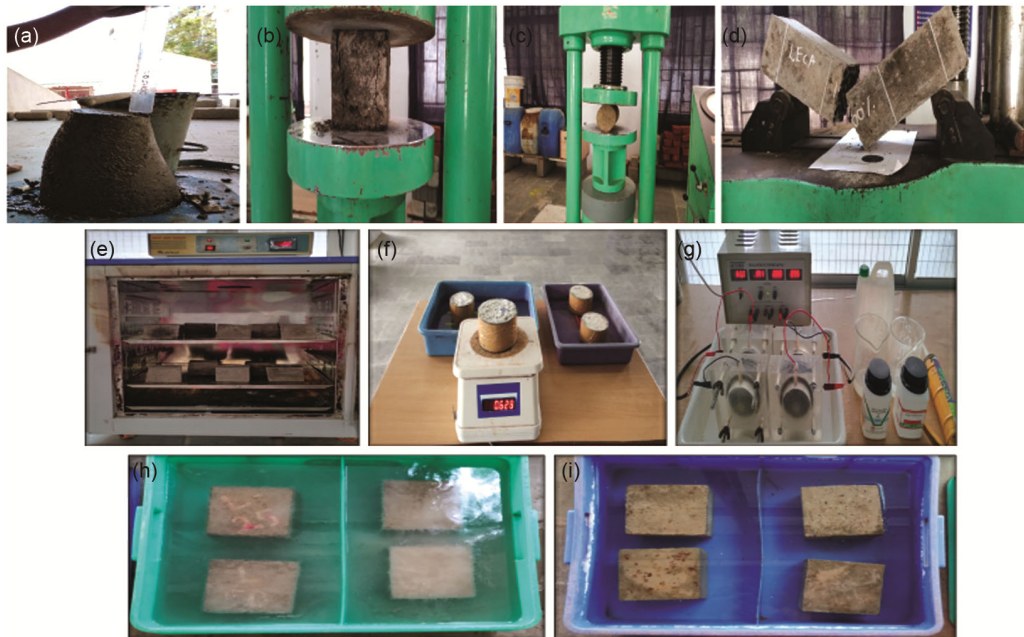
Fig. 5 — Test carried out (a) Slump cone, (b) Compressive strength, (c) Split tensile strength, (d) Flexural strength, (e) Water absorption, (f) Sorptivity, (g) Rapid chloride penetration, (h) Acid attack, and (i) Sulphate attack, for LECA infused concrete.
