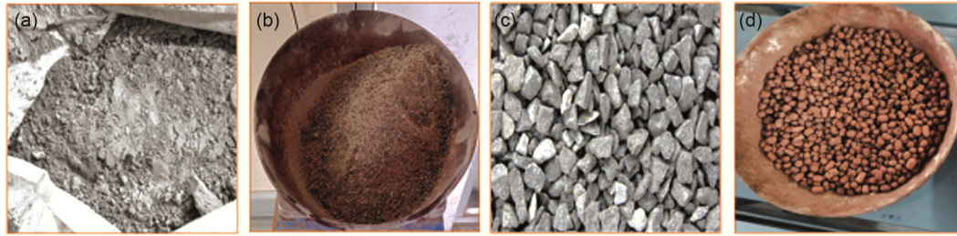
Fig. 2 — Materials used for making LECA infused concrete (a) PPC, (b) M-sand, (c) Coarse aggregate, and (d) LECA.
