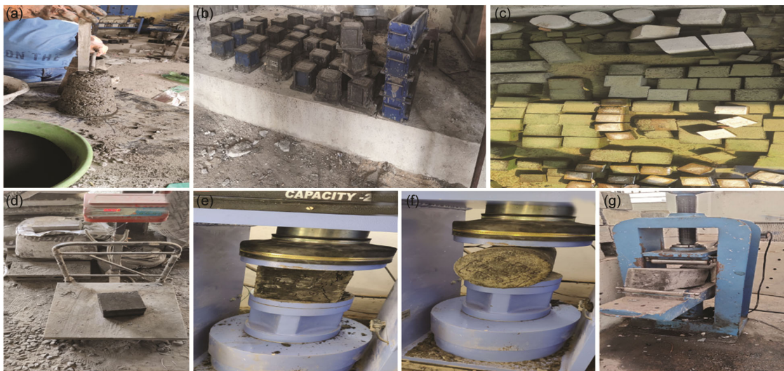
Fig. 23 — Experimental Process (a) Slump test, (b) Preparation of samples, (c) Curing of samples, (d) weight of cubes for density, (e) Cube test on compressive testing machine, (f) Cylinder test on compression testing machine, and (g) Testing of beam on flexural testing machine.
