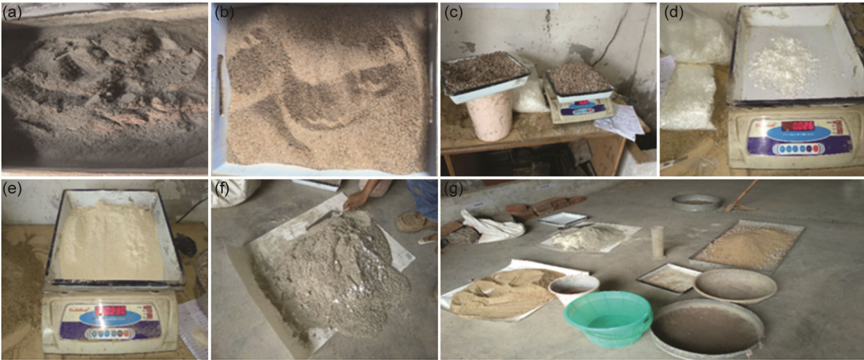
Fig. 5 — Materials (a) Cement (OPC 43 grade), (b) Fine aggregates (FA), (c) Coarse aggregates (CA), (d) Polypropylene fiber (PPF), (e) Metakaolin (MK), (f) Silica fume (SF), and (g) Experimental materials.
