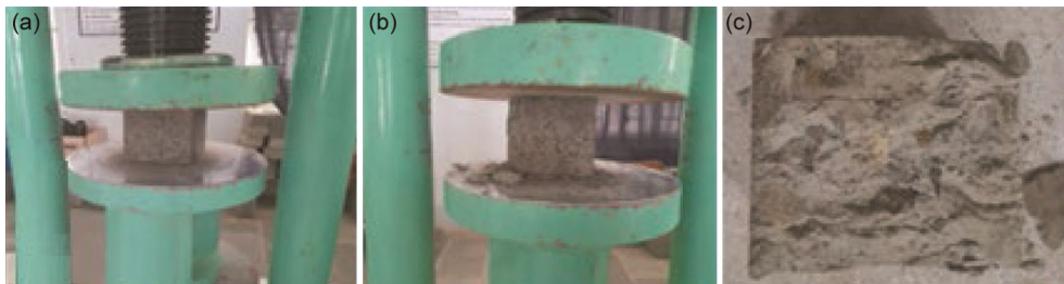
Fig. 6 — (a) Placing of specimen under compression loading, (b) Specimen crushing during loading and (c) Failure specimens after loading.
