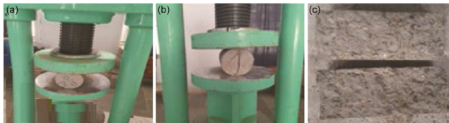
Fig. 8 — (a) Placing of specimen under split tension loading, (b) Specimen crushing during loading and (c) Failure specimens after loading.
