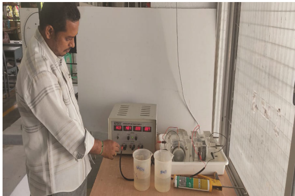
Fig. 15 — RCPT test setup.
