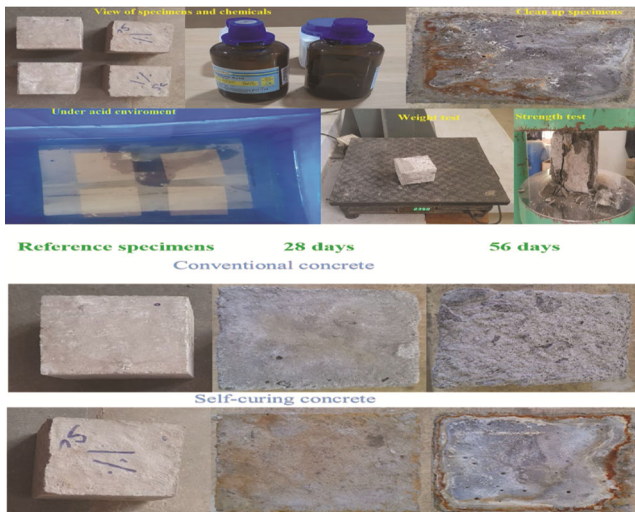
Fig. 17 — Immersion and appearance of specimens in acid resistant test.
