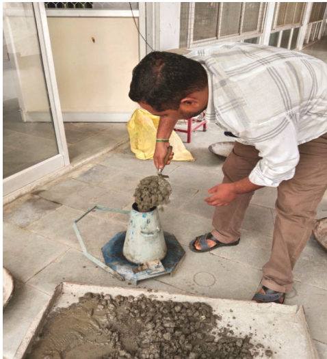
Fig. 4 — Slump cone test.
