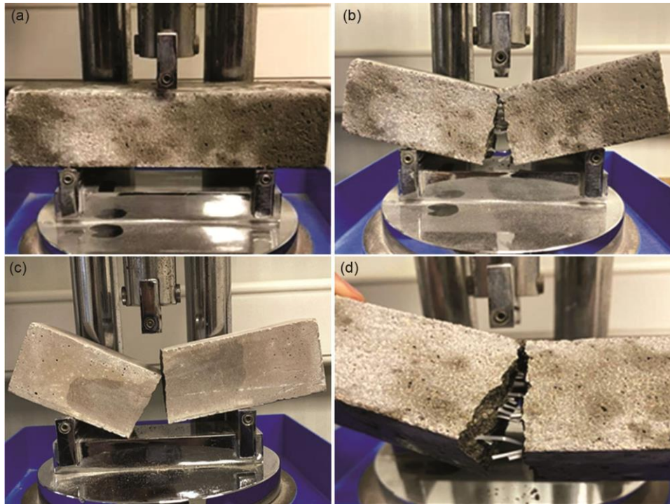
Fig. 3 — Three-point bending testing of specimens
