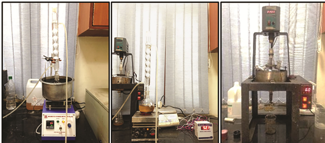
Fig. 3 — Round bottom flask reactors used for biodiesel production.
