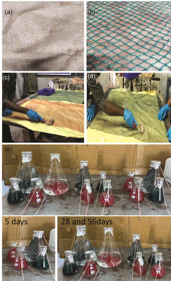
Fig. 1 — a) Uncoated Anchovy fishing net (Red net), (b) Deep sea fishing net (Green net) (c) coating of Anchovy red net (d) coating of green net (e) Dipping of Anchovy and Deep sea net in alkali (NaOH) Solution for 5 days, 28 days and 56 days.
