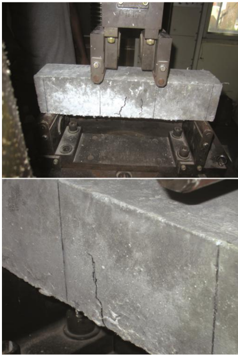
Fig. 26 — Failure of prisms in flexural testing.
