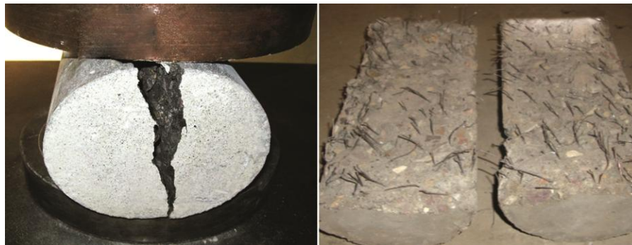
Fig. 25 — Failure of cylinders in split-tensile strength.
