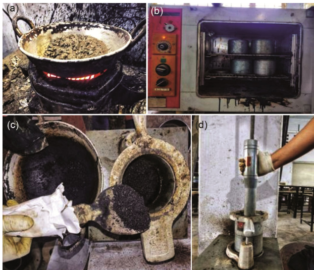
Fig. 2 — Sample preparation process (a) aggregate heating, (b) mould inside the oven, (c) transferring mixture into the mould and (d) hammering.
