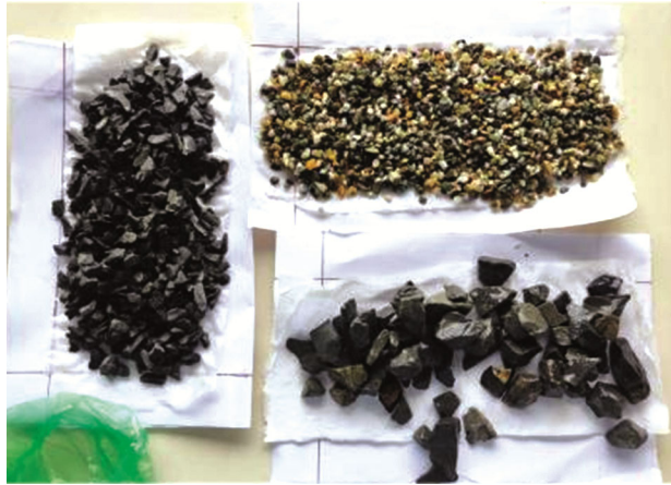
Fig. 3 — Etched coarse aggregates
