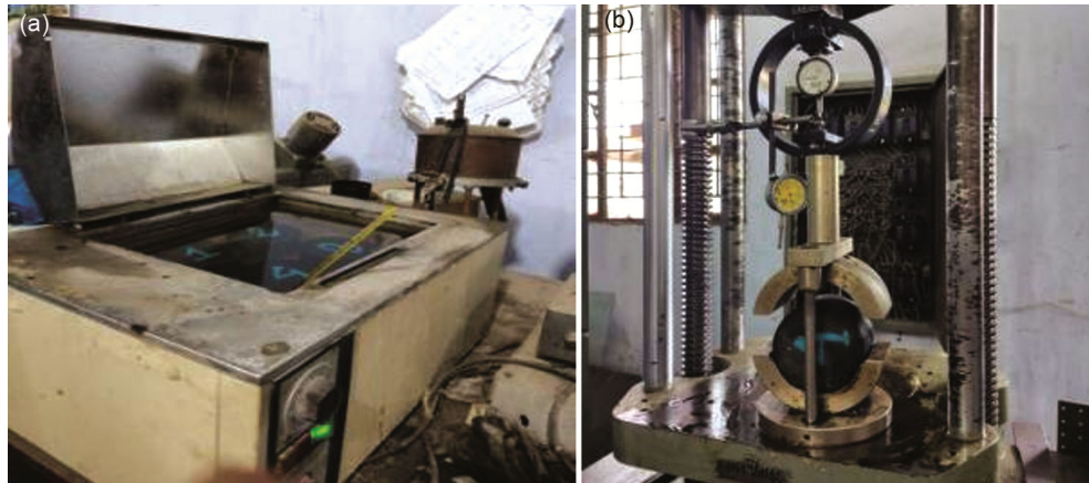
Fig. 5 — Instrument (a) water bath and (b) Marshall testing machine used in the present experiment.
