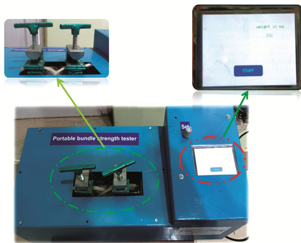
Fig. 5 — Developed portable digital bundle strength tester.
