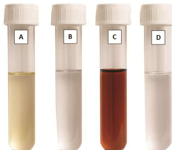
Fig. 1 — Optical monitoring of biosynthesis of silver nanoparticles. (A) Aqueous leaf extract; (B) Silver nitrate solution (AgNO 3 ); (C) Brown colloid, which indicates the formation of green-synthesized silver nanoparticles; (D) Distilled water control. Nanoparticle formation is confirmed by the change of color from light yellow to dark brown.
