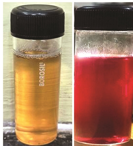
Fig. 1 — Colour Change during phytochemical synthesis of chloroauric acid to ruby red colour.
