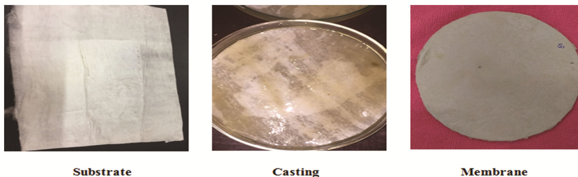
Fig. 5 — Construction of membrane
