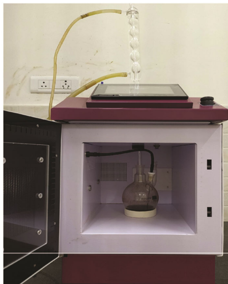
Fig. 1 — Microwave-assisted transesterification reaction setup
