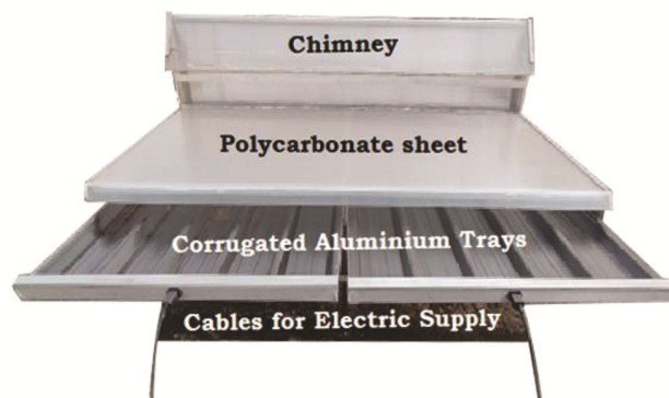
Fig. 2 — Corrugated Electric Solar Conduction Dryer
