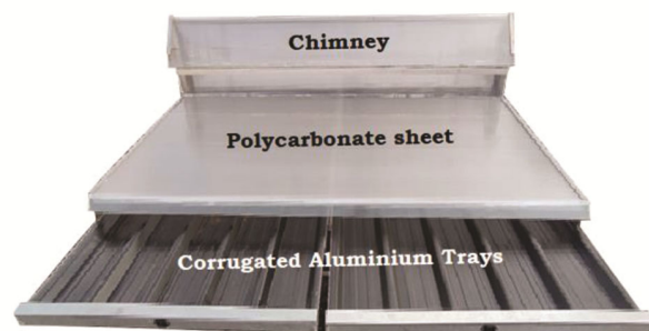
Fig. 3 — Corrugated solar conduction dryer
