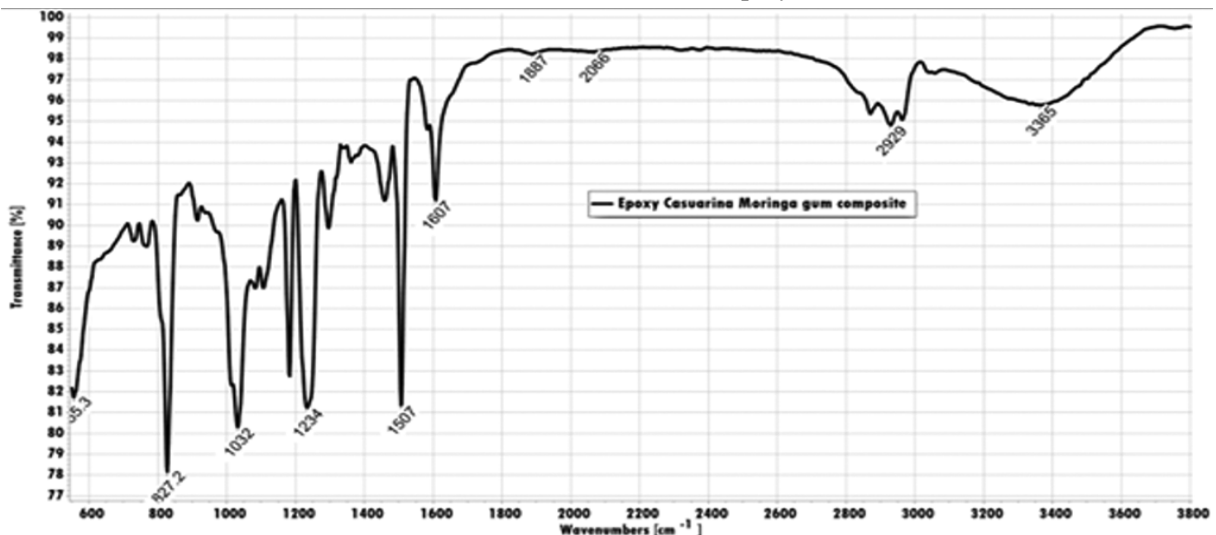
Fig. 1 — IR spectrum of Moringa gum + Casuarina epoxy composite
