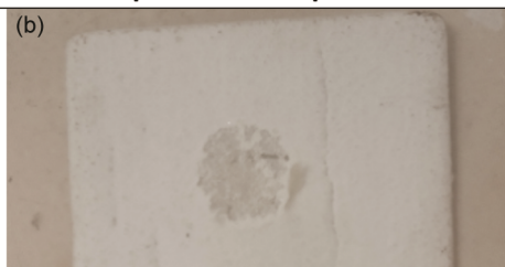
Fig. 4 — Pull off test of samples (a) without and (b) with fire retardant
