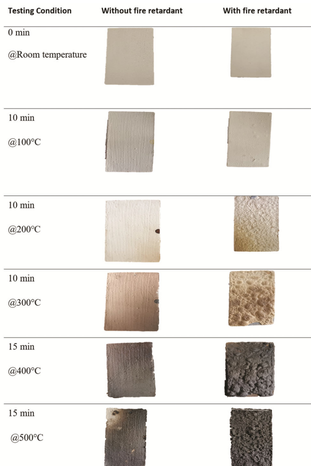
Fig. 6 — Furnace test results
