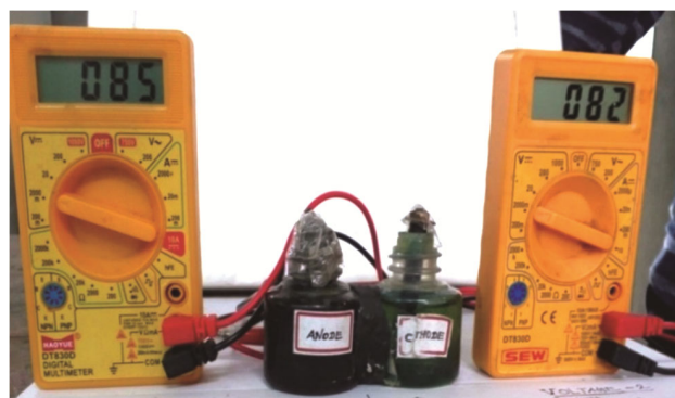
Fig 1 — Experimental setup and operational configuration of the MFC
