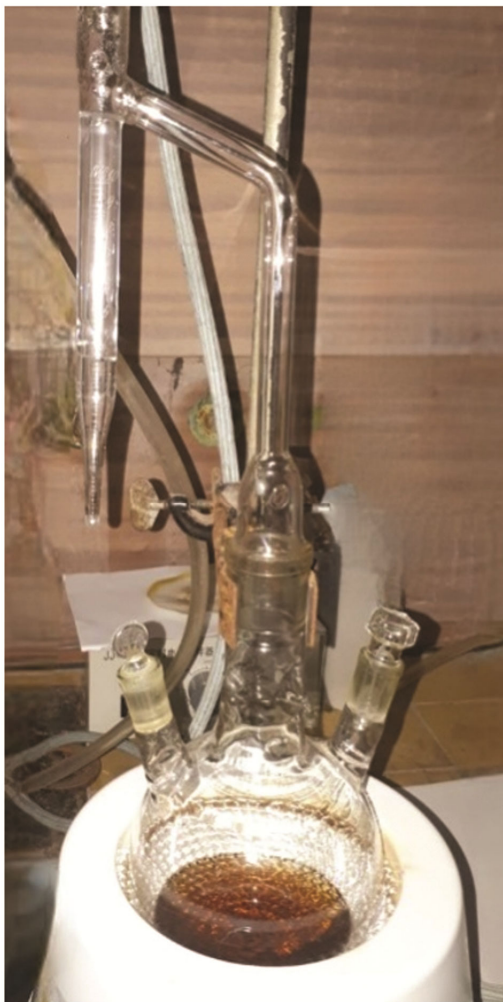
Fig. 2 — Set-up for the preparation of the glycol acetal
