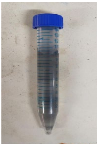
(b) Synthesized hybrid nanofluid (0.005 volume fraction)
