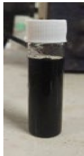
(c) Synthesized hybrid nanofluid (0.03 volume fraction)
