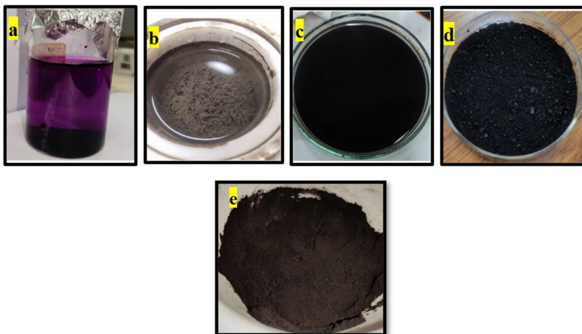
Fig. S1 — Photographs of (a) precursor ( \text{KMnO}_4 ), (b) during autoclave (hydrothermal process), (c) washed and filtered, (d) vacuum-dried sample and (e) \text{MnO}_2 -enriched urea nano fertilizer
