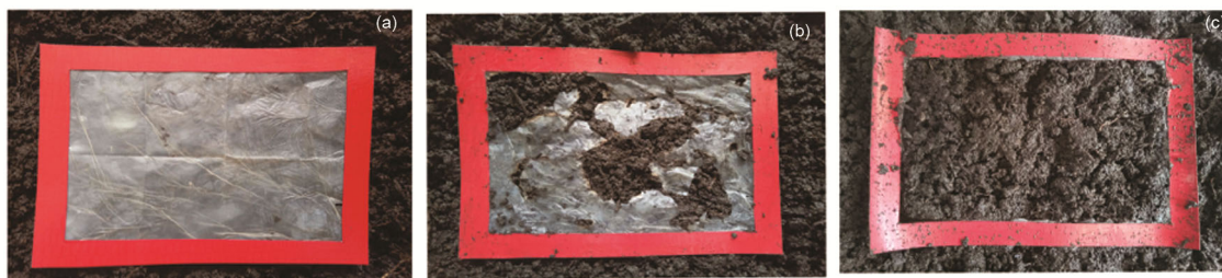
Fig. 8 — Degradation process of the BC microfilter inside humus soil: (a) beginning day, (b) 2 weeks later and (c) 4 weeks later
