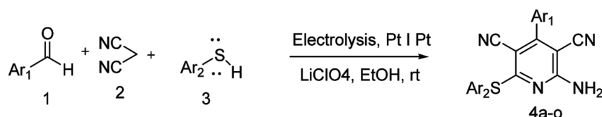
Scheme 1 — Electrocatalytic pathway for synthesis of highly substituted pyridine
