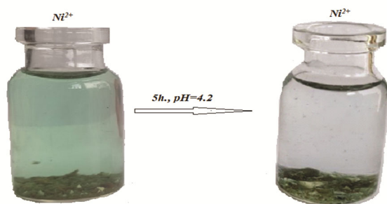
Fig. 4 — Sorption process of FD-EXG polymer sorbent in Ni(II) salt solution
